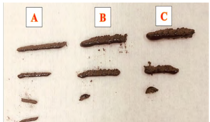
Fig. 24: Samples of 2D printed samples of regolith simulants
